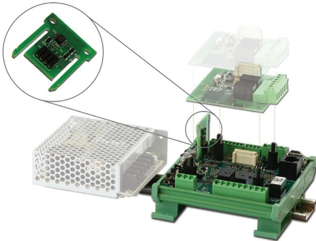
The iCon-2 electronic card checks the electronic control actions, the valve conditions and the ride comfort. Travel curves are recorded in the electronic system. During operation, the travel curves for that particular elevator are optimized by the learning algorithm iTeach.
