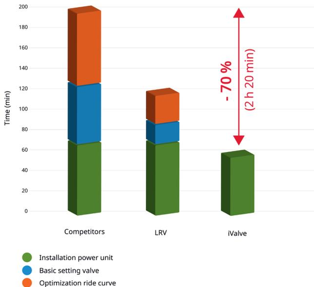
Quick commissioning - The iValve scores points mainly by eliminating the basic valve settings and by optimizing the travel curve.
