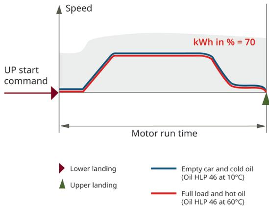
Perfect travel curves under all conditions - The iValve lift-control valve from Bucher Hydraulics automatically compensates for varying loads and oil temperatures.
