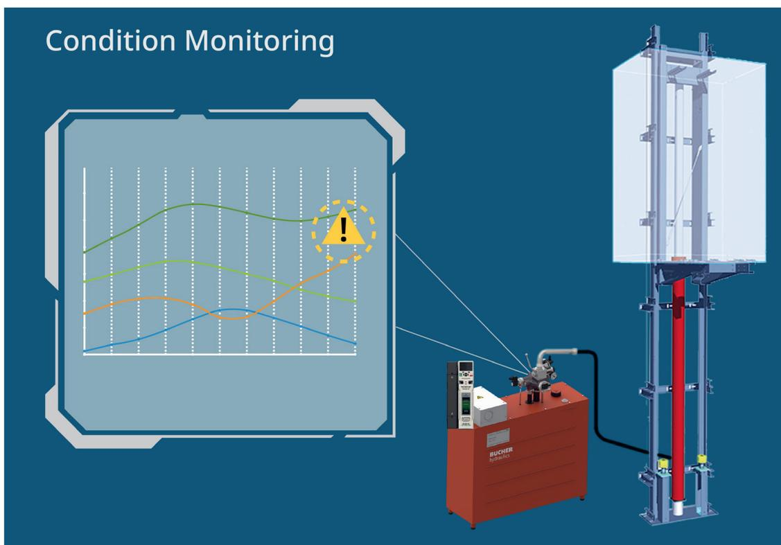
The future has begun - The iValve from Bucher Hydraulics, in conjunction with the iCon-2 controller, provides data for predictive maintenance that helps prevent breakdowns.
